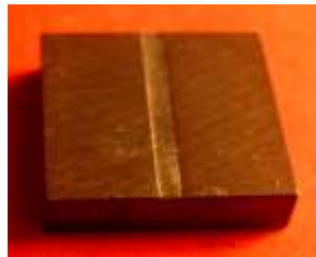
Fig.3 A typical impression specimen after test.
